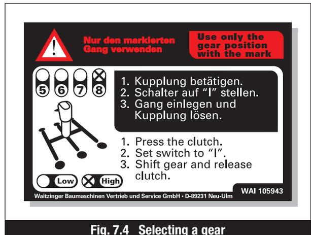
Fig. 7.4 Selecting a gear
