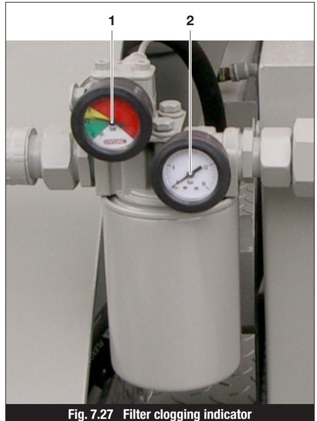
Fig. 7.27 Filter clogging indicator
