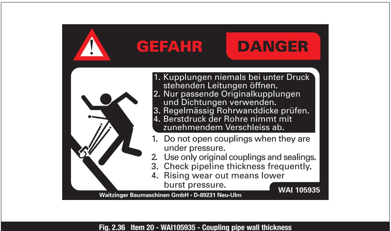
Fig. 2.36 Item 20 - WAI105935 - Coupling pipe wall thickness
